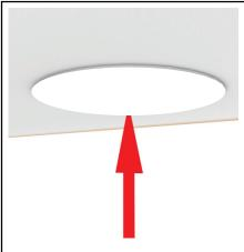
Once clips have been folded up, push panel up flush to the ceiling, Clean off any fingerprints left behind.
