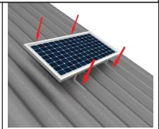
Attach brackets to the roof with roof screws. Seal under the screws and bracket. Run cable under ridge cap and into roof cavity.
